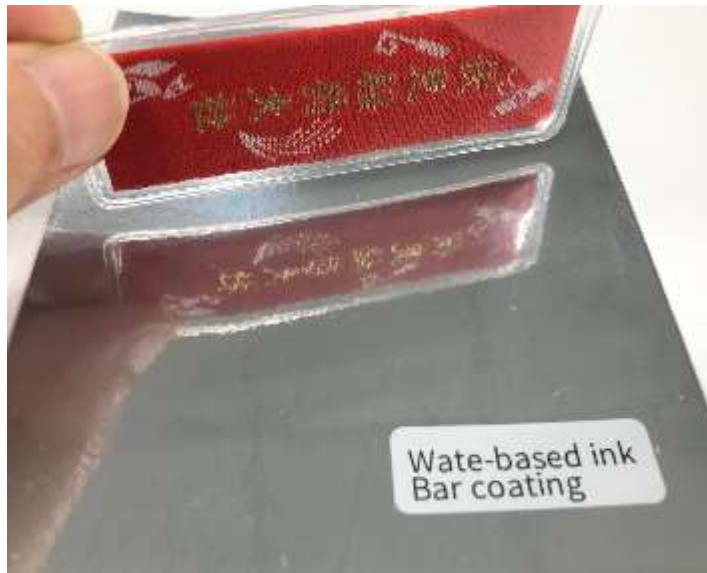
Bar-coated sample of water-based ink
