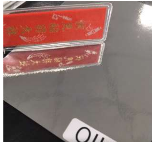
Bar-coated sample of UV curing ink
