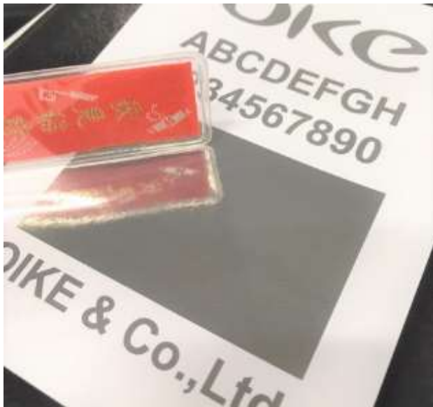
Inkjet printed sample of LeafPowder® In ink
