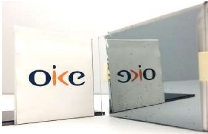
Spin coated sample of LeafPowder™ Indium dispersion
