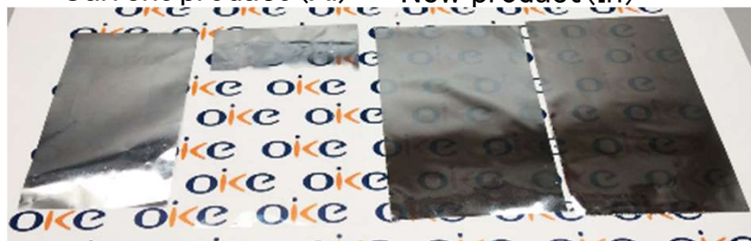
before after before after 60°C water × 1month stability test result (deposited film)
