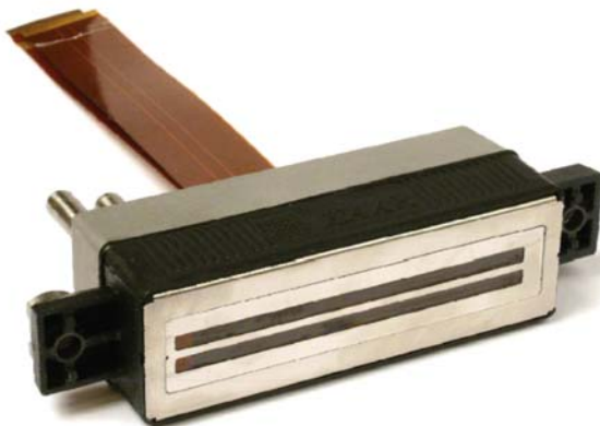
Figure 3. The Xaar1001 printhead with two rows of actuators provides 1000 active nozzles at 360 dpi effective nozzle pitch.
